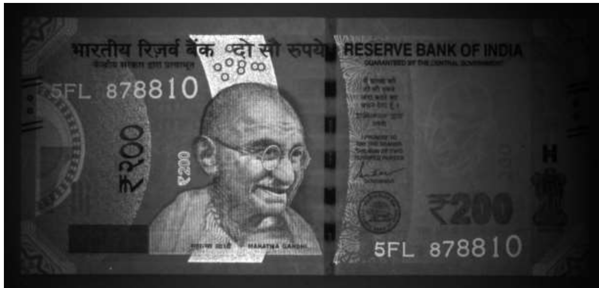
Fig 13: Obverse side of Rs. 200 denomination Indian bank note under IR light
