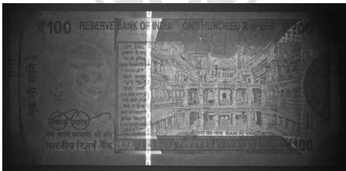
Fig 18: Reverse side of Rs. 100 denomination Indian bank note under IR light
