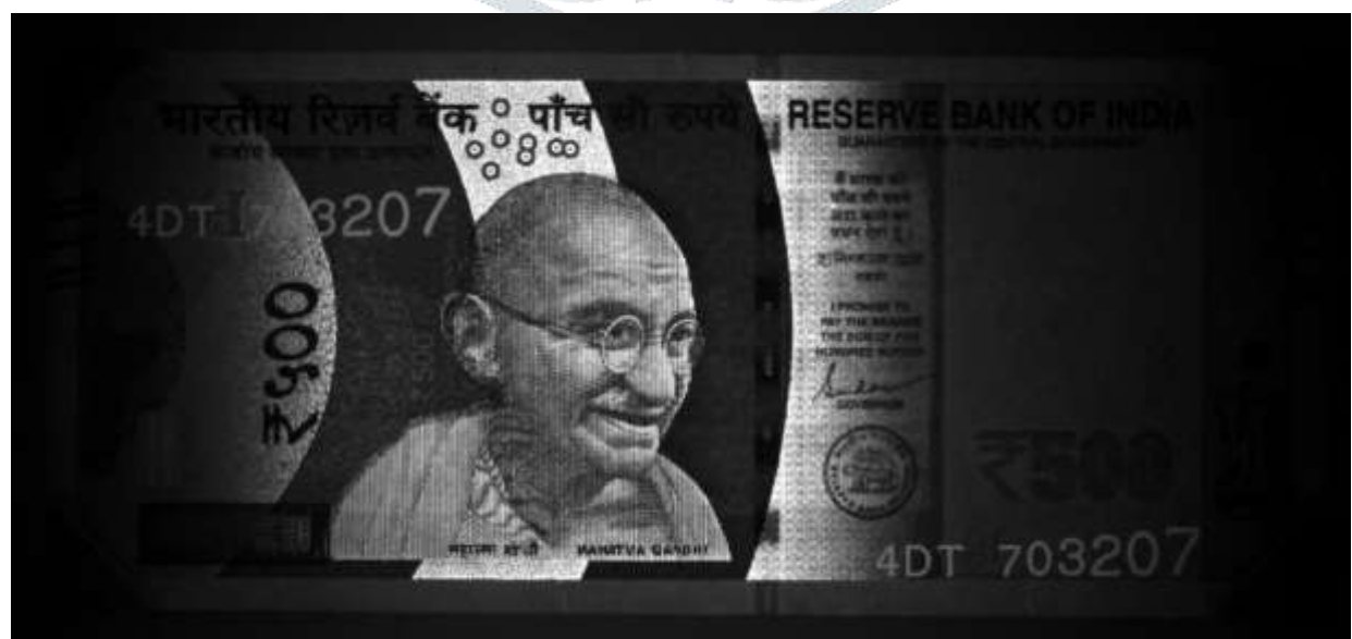
Fig 9: Obverse side of Rs. 500 denomination Indian bank note under IR light
