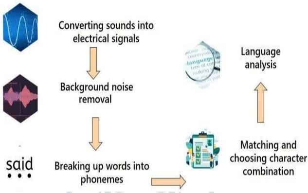
Fig 10: Algorithm Flow
