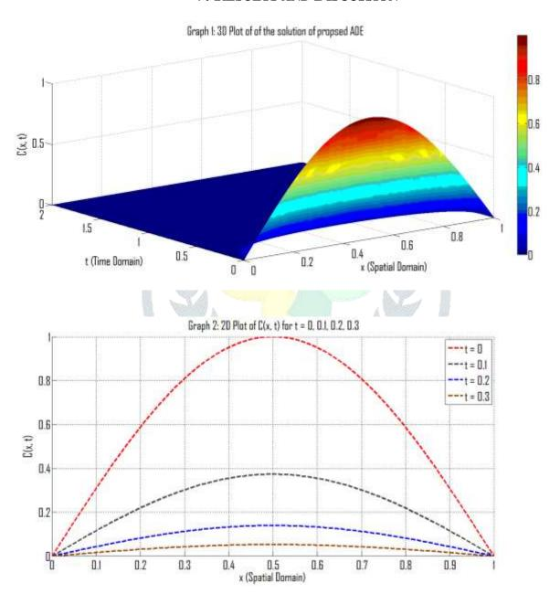
The 3D plot in graph (1) depicts the solution of a proposed Advection-Diffusion Equation (ADE) over a time-space domain. The horizontal axes represent the spatial domain (x) and the temporal domain (t), while the vertical axis corresponds to the solution C(x,t), which is likely a concentration profile. The color gradient indicates the magnitude of C(x,t), with blue representing the lowest values and red the
