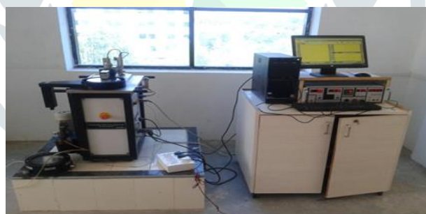
Fig. 4.1.1 Photograph of experimental set up (Tribometer TR-20LE).
