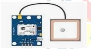
The NEO6M-V2 GPS module is used for real-time location tracking of the borewell. It connects to satellites to retrieve accurate latitude and longitude coordinates, which are then transmitted to the ESP8266 for display on a web server. The GPS data is crucial for rescue teams as it helps pinpoint the borewell location during emergencies. This module operates on a 3.3V power supply and communicates with the microcontroller via serial UART, ensuring seamless integration with the system
