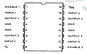
The L293D H-Bridge driver is a motor driver IC used to control the loader arm mechanism responsible for automatic borewell closure. It receives commands from the CH340 microcontroller and regulates the movement of the DC motors that operate the loader arms. This IC enables bidirectional motor control, ensuring smooth and precise operation of the closure mechanism.
