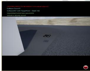
The image shows a drone simulation in AirSim, where the UAV is successfully armed and controlled via API. The collision count remains zero, indicating safe navigation through obstacles, while Unreal Engine prompts lighting issues.
