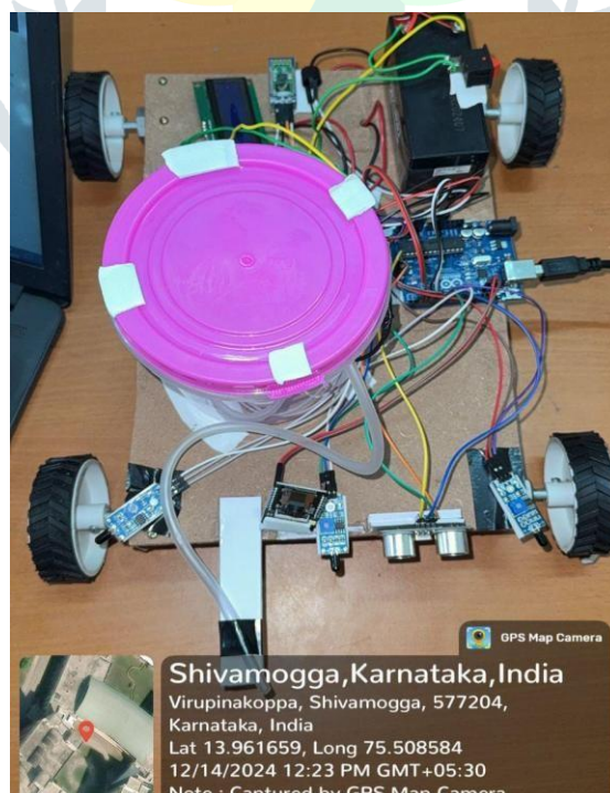
Fig.2. Fire Combat System Using Arduino model
