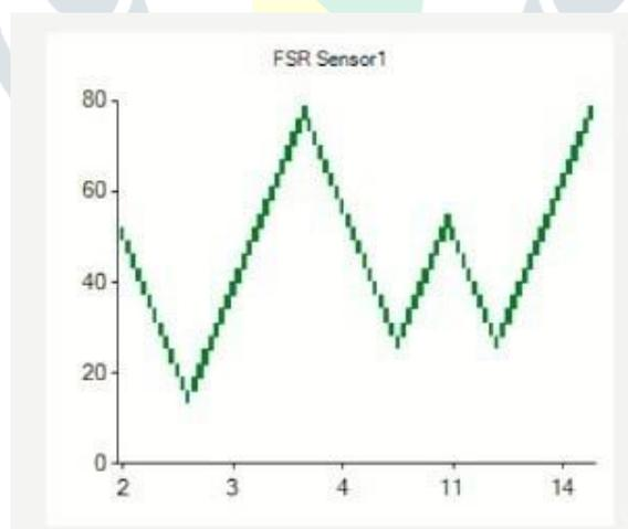
A Force Sensitive Resistor (FSR) is a type of sensor that changes its resistance based on the applied force or pressure. It consists of a conductive polymer that exhibits a decrease in resistance as more pressure is applied. In the graph, the y-axis represents force, while the x-axis corresponds to time or another relevant variable. The upward peaks signify instances of increased force application, whereas the downward dips indicate periods of reduced or no applied pressure.
