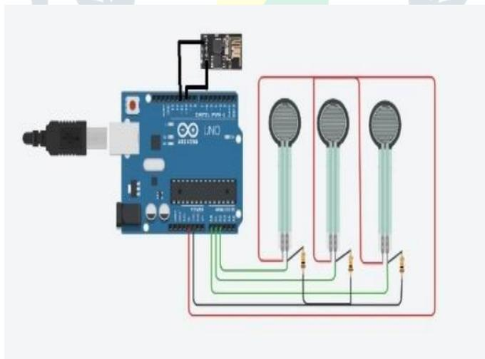
pressure reduces the resistance of the FSR, leading to a corresponding change in the voltage that the analog input needles of the Arduino (A0, A1, A2).
