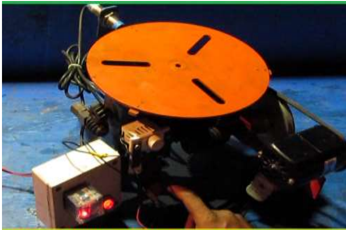
Automatic -Multi Axis Welding Positioner Continuous / Staggered Welding ( 60 , 90 , 120 , 180 Degree) Auto Stop , Variable Speed Variable Inclination ( 0 to 45 degree---Self Locking Table
