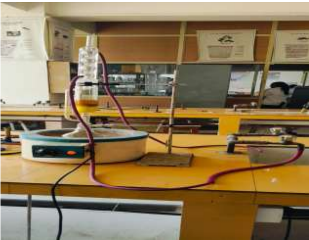
Fig.no.2 Soxhlet extraction of powder of curcumin
