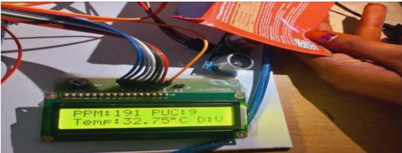
**Fig.5.4: Counting Push-ups using Ultrasonic Sensor**
