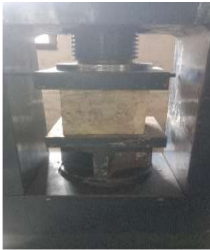
Fig-3: compression test of concrete cube
