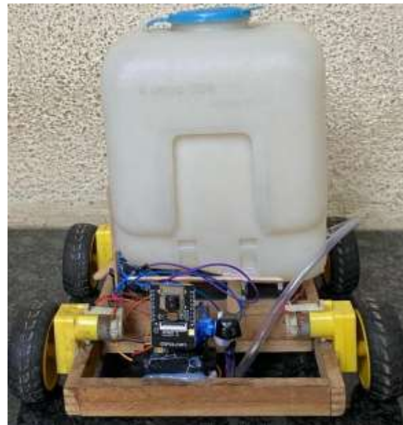
Figure 2: Prototype Model of the firefighting robot/testing phase
