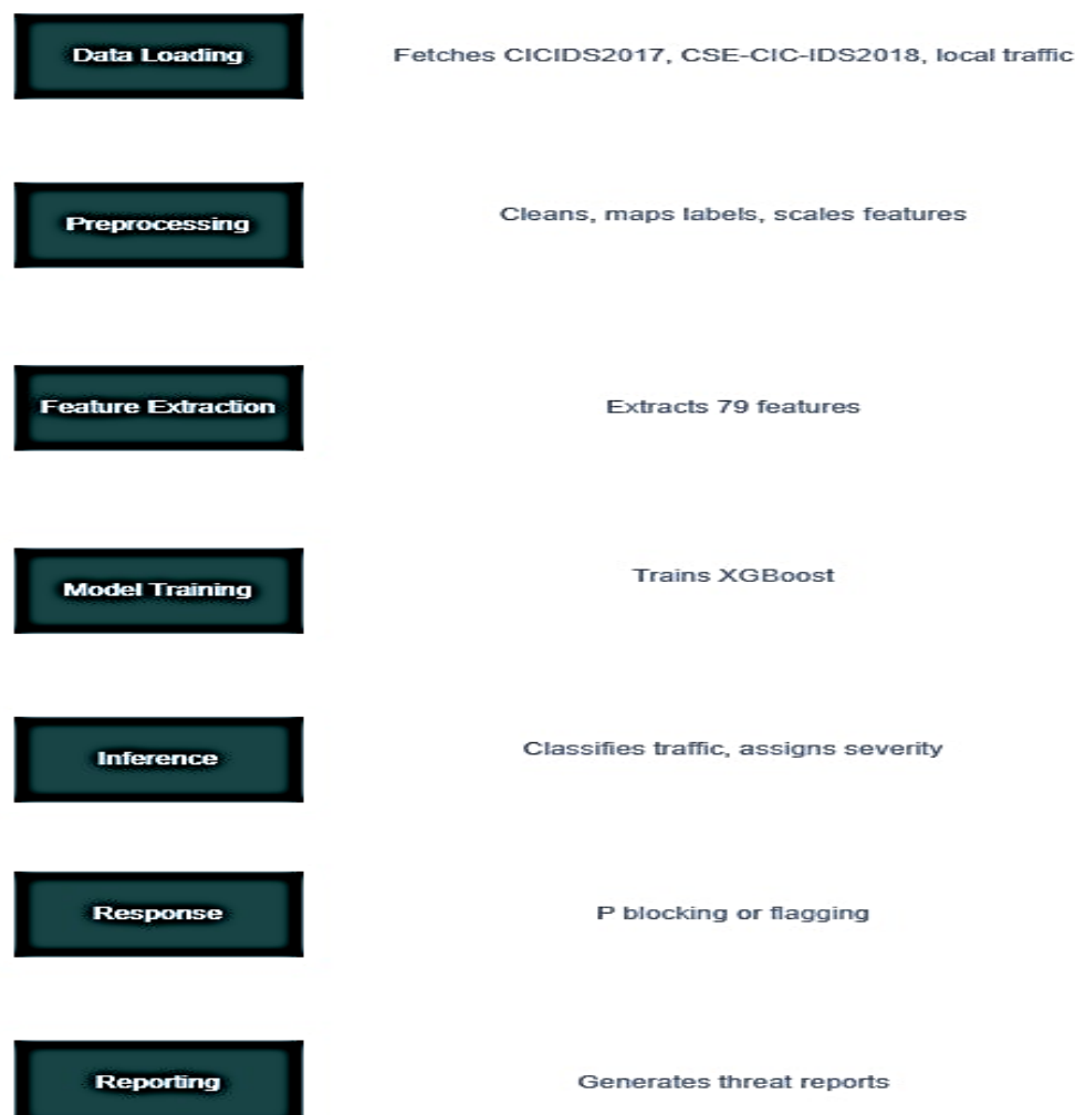
Figure 6.1: Data Flow Diagram showing data loading, preprocessing, training, inference, response, and reporting
