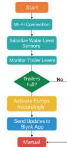
Figure 3: Flowchart for Waste Management System Operation
