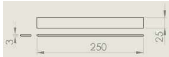
Figure 4: Line diagram for compression test specimen as per ASTM C1275 Standards.
