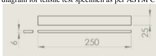
Figure 3: Line diagram for flexural test specimen as per ASTM C1275 Standards.
