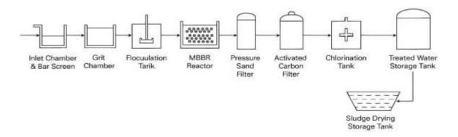
Figure 1: Process Flow Diagram
