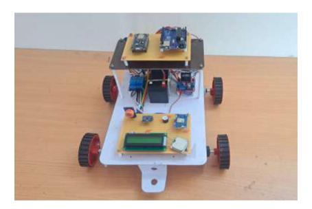
Figure shows a prototype demonstrates a smart vehicle system with alcohol detection, GPS tracking, and IoT monitoring. It uses an Arduino UNO, MQ-3 sensor, GPS module, and NodeMCU to detect alcohol levels, track location, and transmit data online. The motor is controlled via relay based on sensor input, enhancing road safety by preventing vehicle operation under intoxication
