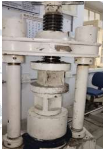
Fig 5: compressive strength test
