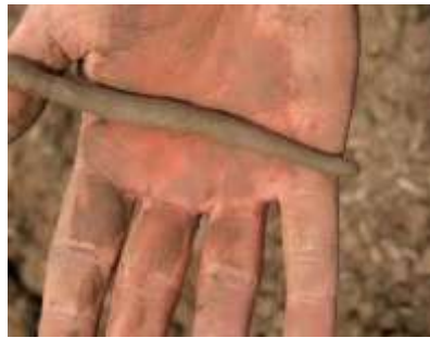
Fig 6.5. Plastic limit soil sampl
