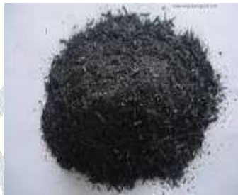
Fig 5.3. Sugarcane bagasse ash
