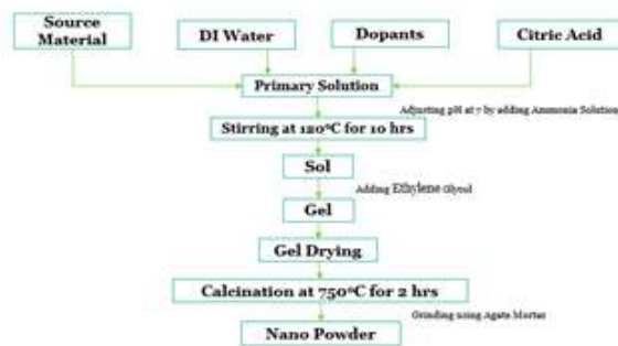
Figure 1 Flow chart of NiO and Zn–NiO nanoparticles
