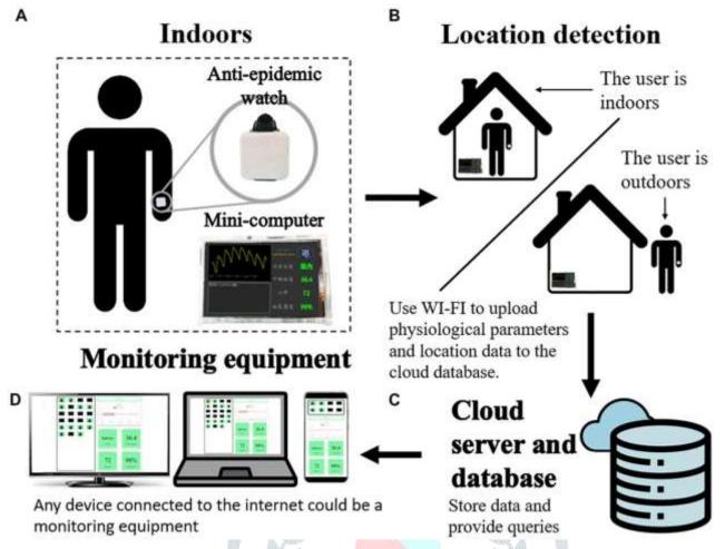
IoT-based wearable health monitoring system architecture using anti-epidemic watch, cloud server, and multi-device access for indoor/outdoor location detection.
