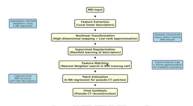
Fig:- Block Architecture of MRI to CT prediction via nonlinear local Descriptors
