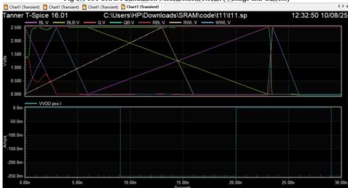
Fig 18. 11T SRAM Waveform Output – Voltage and Current Characteristics
