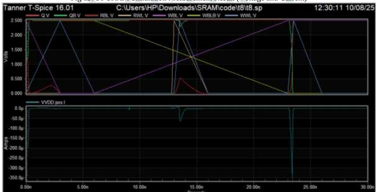
Fig 14: 8T SRAM Waveform Output – Voltage and Current Characteristics
