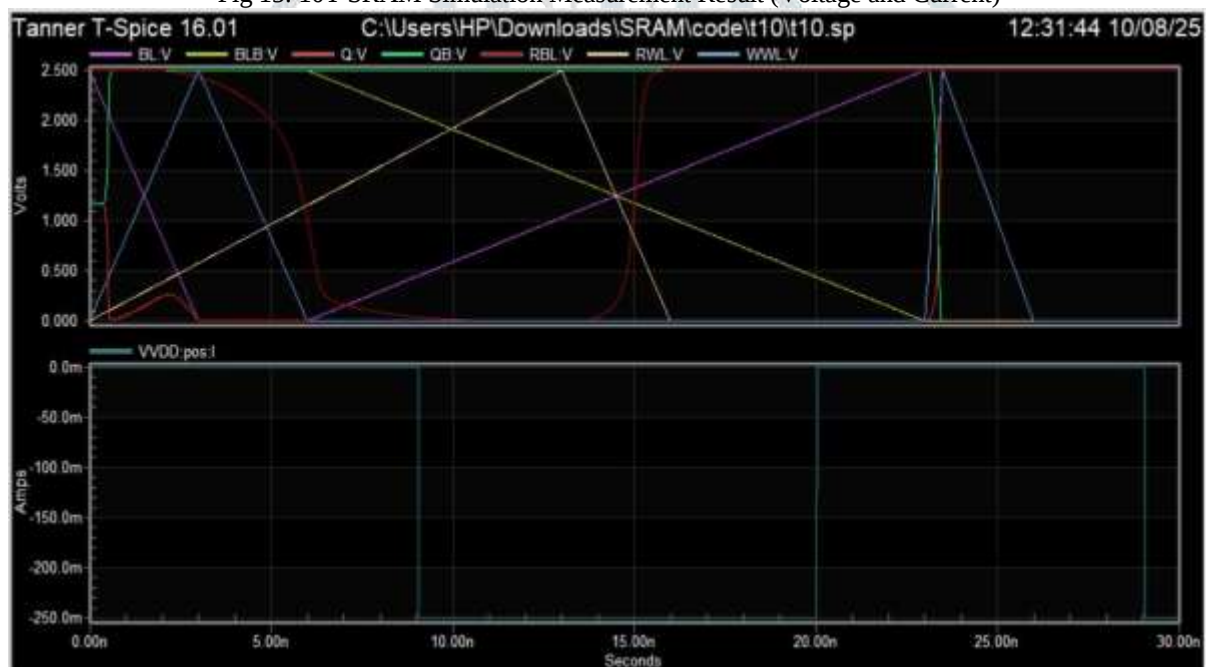
Fig 16. 10T SRAM Waveform Output – Voltage and Current Characteristics
