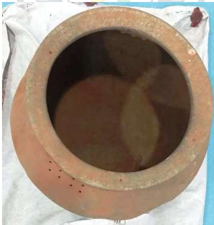
Fig 5. Pot having height 12 in. and inner diameter 9 in.
