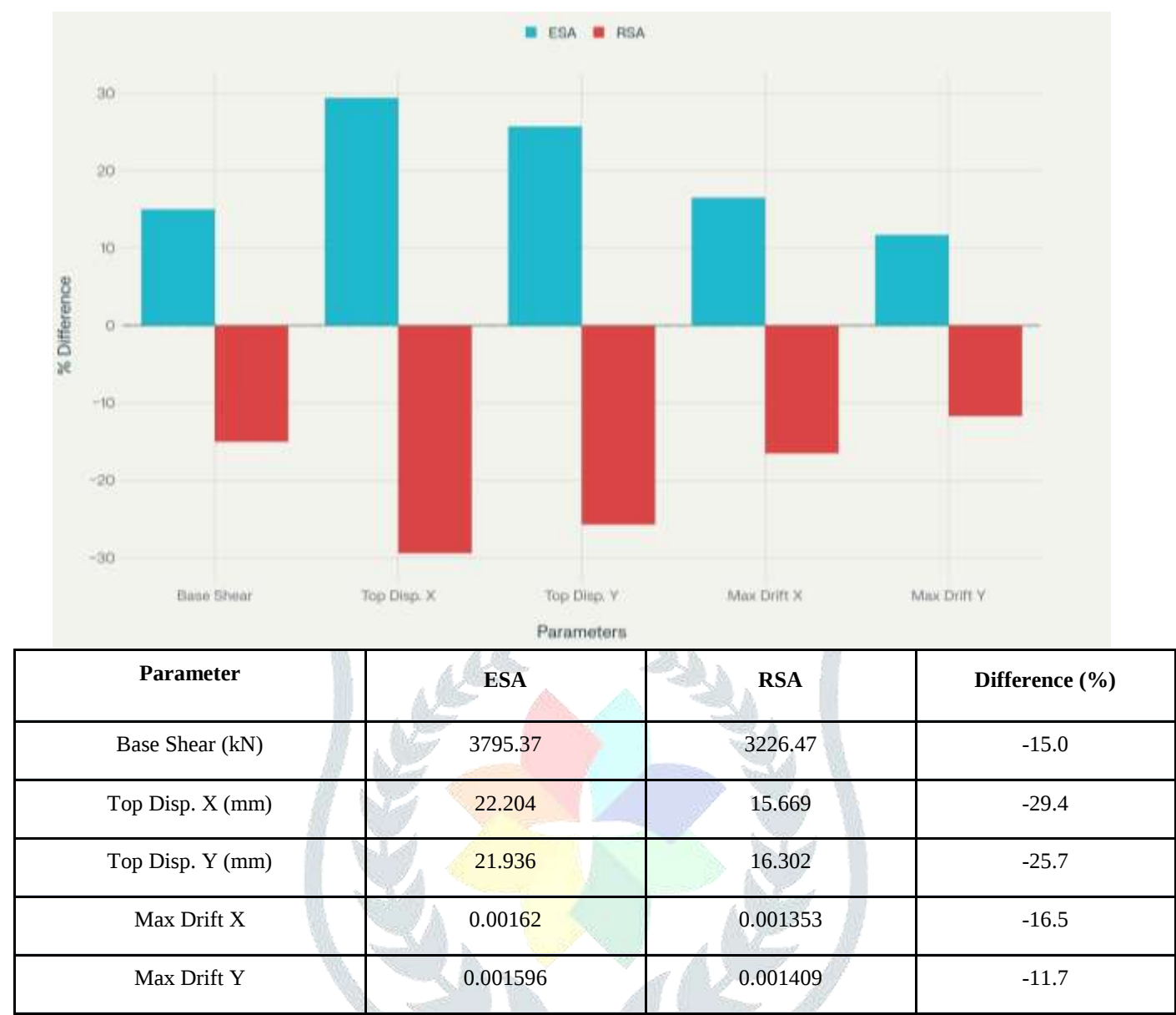
Figure 11: Percentage differences showing ESA consistently overestimates structural response compared to RSA across all key parameters.
