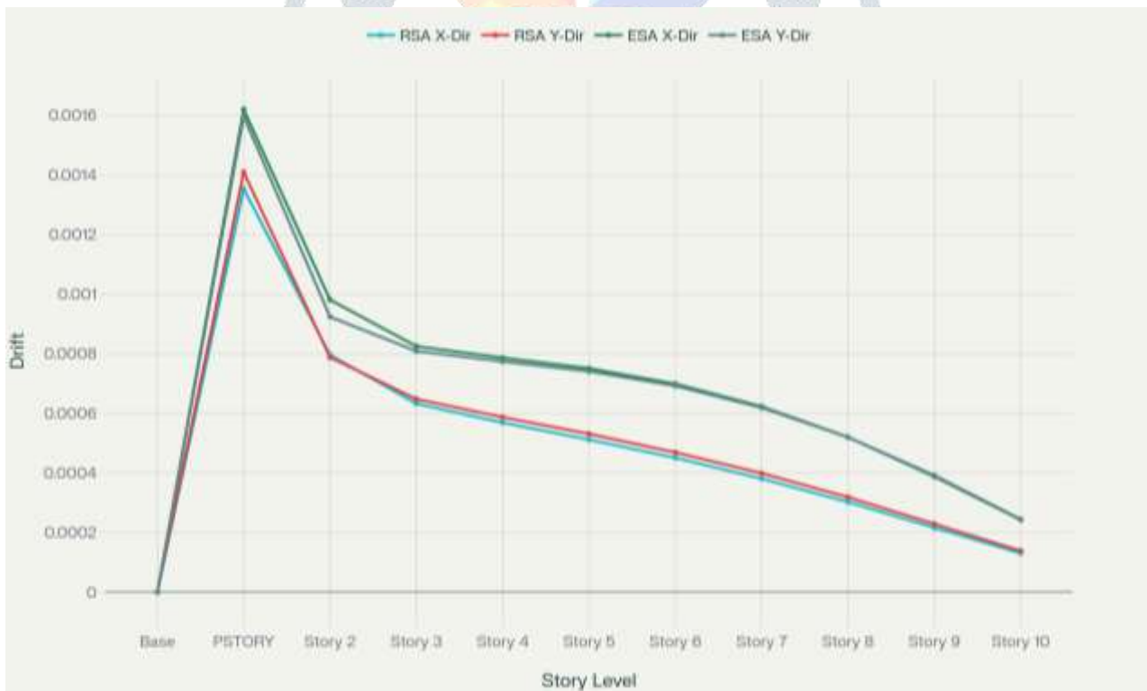
Figure 8: Story drift comparison showing ESA overestimates drift values compared to RSA, with maximum drift at PSTORY level in both methods
