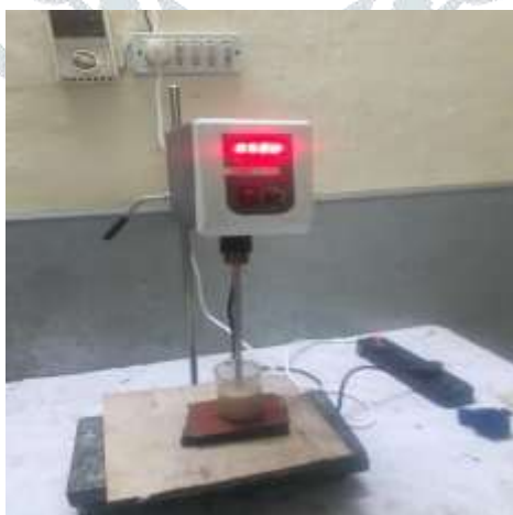
Figure 2.3: Mixing of filler with Polyester resin using Mechanical stirrer
