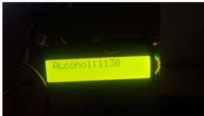
Fig. 5. Alcohol level detection displayed on LCD screen.
