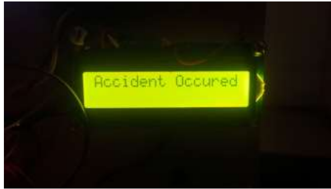
Fig. 6. Accident detection alert displayed on LCD screen.
