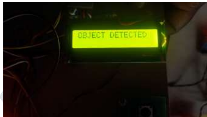
Fig. 7. Obstacle detection warning displayed on LCD screen.
