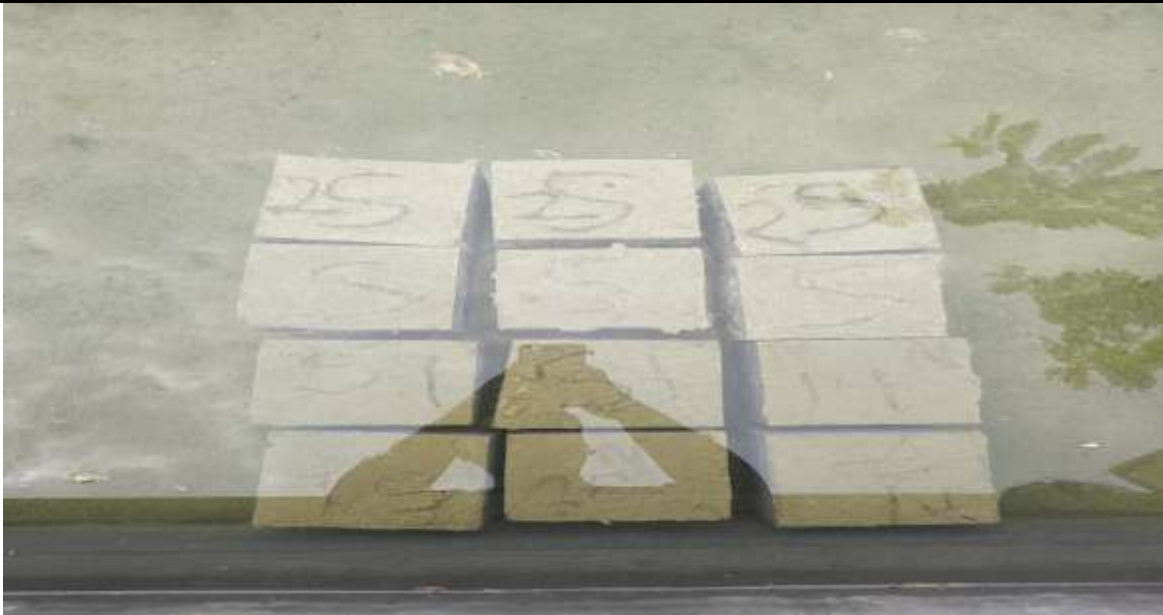
Figure 2. Curing of concrete cube specimens in a water tank
