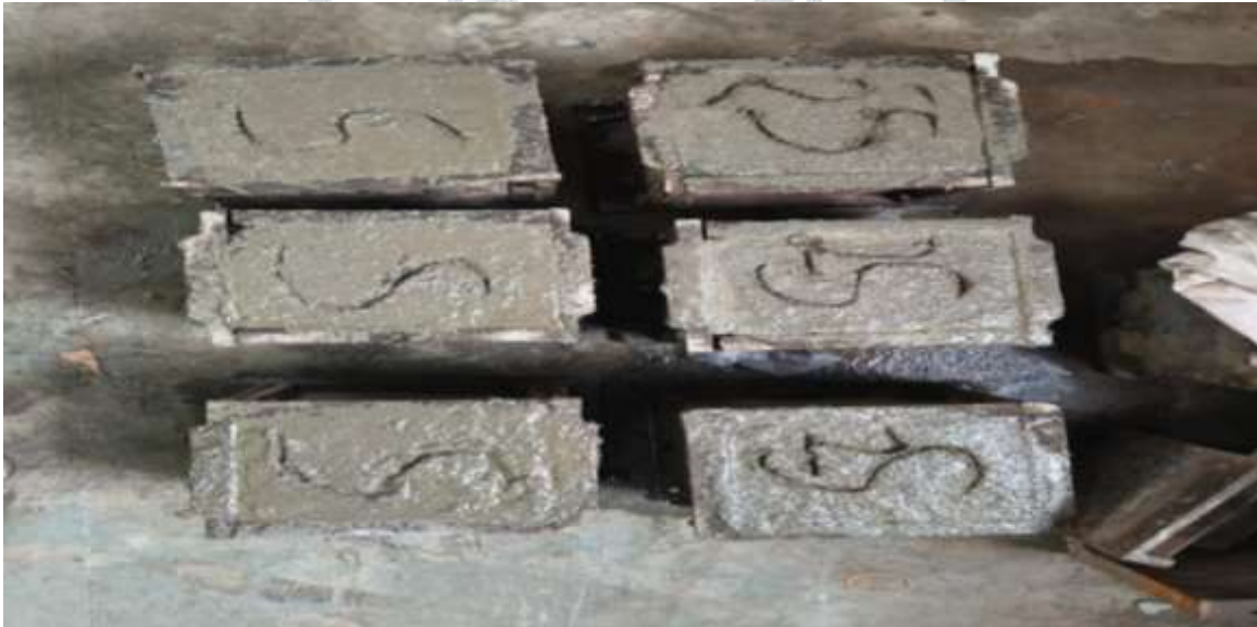
Figure 1. Fresh concrete filled into 150×150×150 mm cube molds during casting and marking
