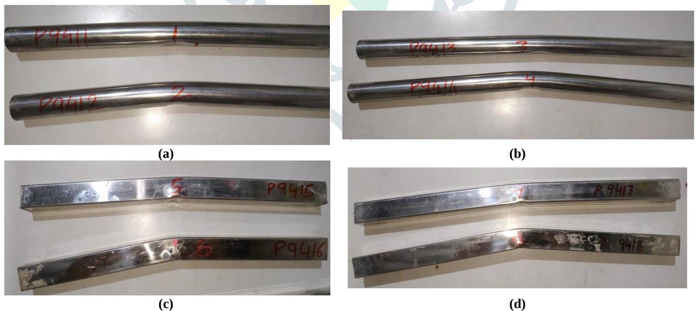
Fig 3: CFST Specimens after compression test (a) circular specimens with L/D as 13 (b) circular specimens with L/D as 18 (c) rectangular specimens with L/D as 13 (d) rectangular specimens with L/D as 18
