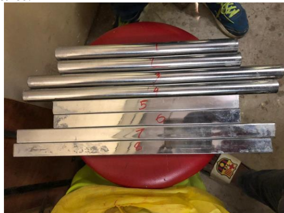
Fig 2: CFST Specimens before compression test
