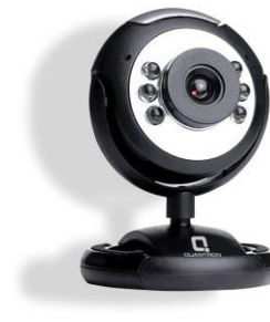
Fig. 2. USB Webcam (visual sensor for frame capture)
