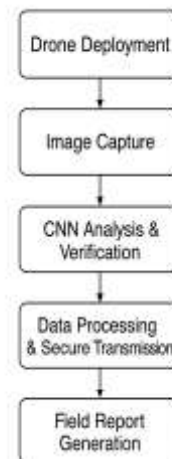
Fig. 2. Workflow of the proposed Agri Vision Drone using CNN
