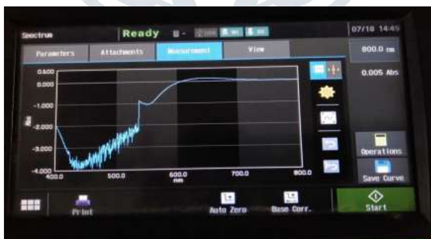
Figure 7: Zero derivative spectrum of Ethambutol hydrochloride conc. 90µg/ml
