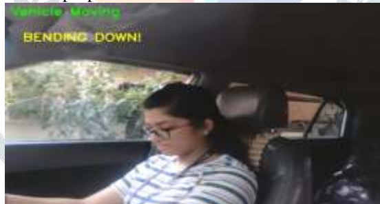
Figure 10: Alert triggered as driver bends down while vehicle is in motion. If the driver bends down or looks away from the road, the system detects this unsafe movement and activates an alarm to regain the driver's attention.
