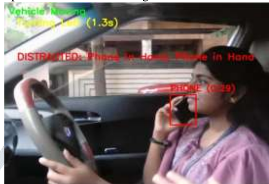
Figure 13: Alert triggered as driver uses phone in right while driving.
