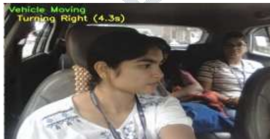
Figure 11: Alert triggered as driver turns right while distracted. If the driver turns right and continues to be inattentive for more than 3 seconds, the system issues a warning alarm. This helps the driver regain focus and avoid potential road hazards.
