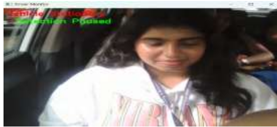
Figure 7: Driver's eyes closed, but no alarm triggered since the vehicle is stationary. When The Vehicle is in Movement:
