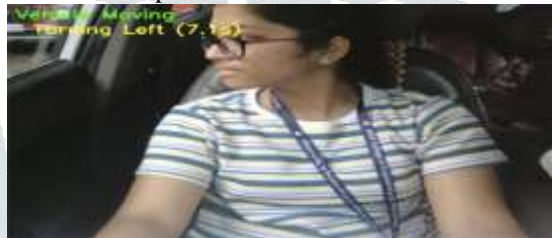
Figure 9: Alert triggered as driver turns left while distracted. When the driver turns left and remains distracted for over 3 seconds, the system identifies unsafe behavior. An alert is activated to remind the driver to stay focused and maintain proper lane control.
