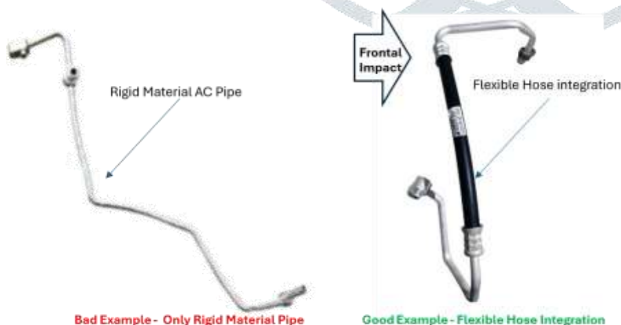
Fig. Flexible Hose Integration in AC Pipe to absorb Frontal low -speed Crash impact energy
