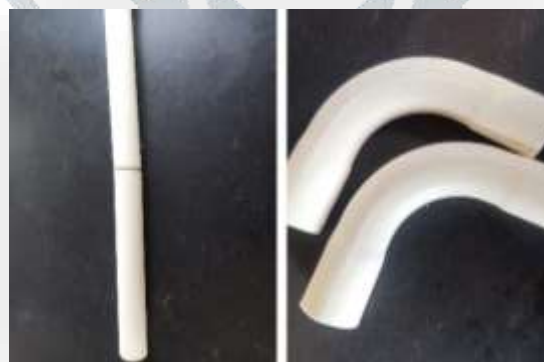
Figure 8: Bent PVC pipe of dia. 1" before and after process
