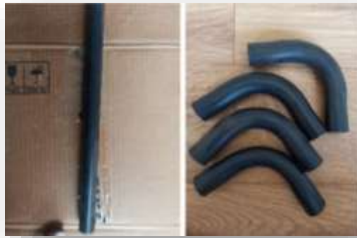
Figure 6: Bent PVC pipe if dia. 1.5" before and after process
