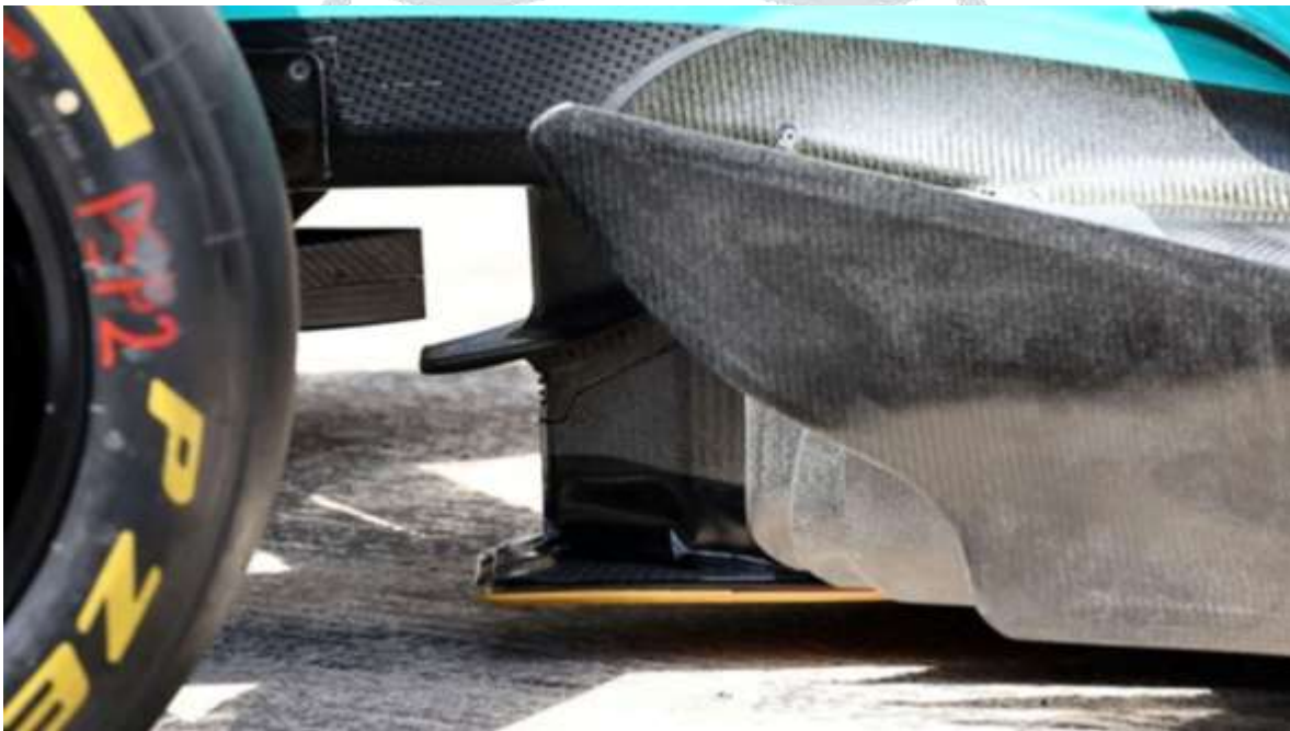
Front floor fillet connecting the front floor bib and the main floor panel as seen on the 2024 Mercedes AMG W16
