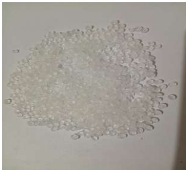
Fig. 3: Polypropylene H350FG Matrix Material Pallets (a), FTIR spectra of Epoxy before and after cross linking (b).
