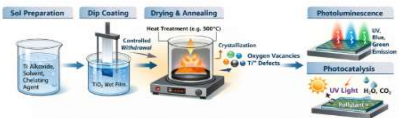
Figure 1: Schematic of the sol-gel dip-coating process, defect formation, and resulting functional properties of TiO 2 thin films.
