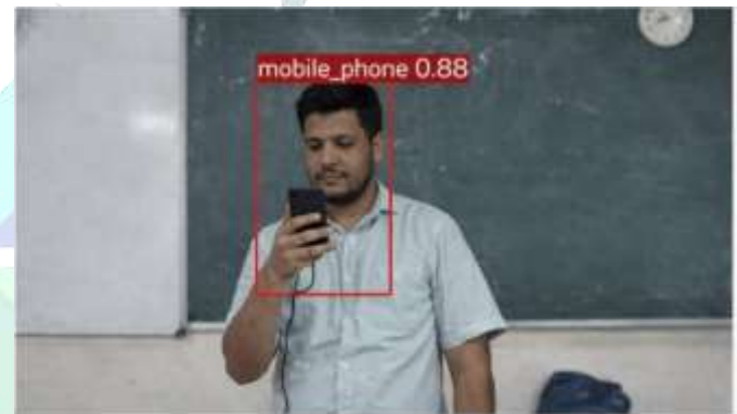
Fig. B. Sample output showing mobile phone detection using YOLOv5 in a restricted environment.
