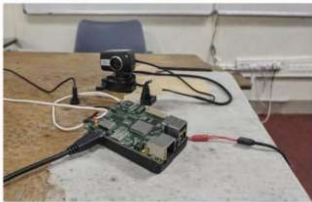
Fig. A. Experimental setup with Raspberry Pi 5 for real-time mobile phone detection.
