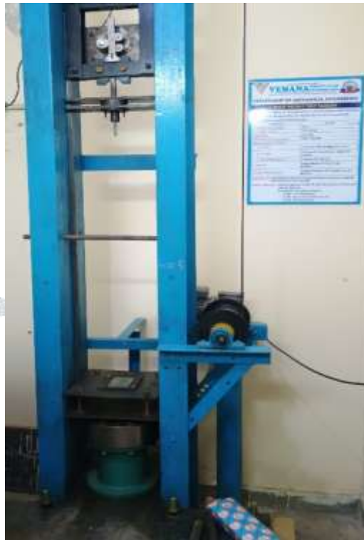
Fig 5. Drop weight impact test facility
