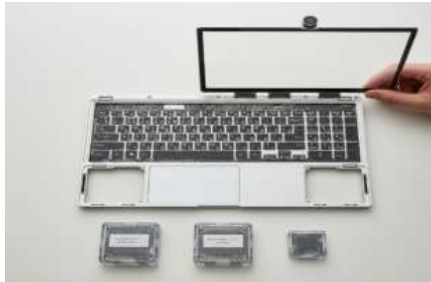
Figure 2.1: Visionary of Multifunctional Custom Upgradable Board (MCUB)
