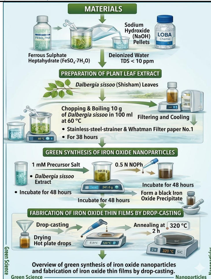
Figure 2: Green synthesis and thin-film fabrication workflow of iron oxide nanoparticles
