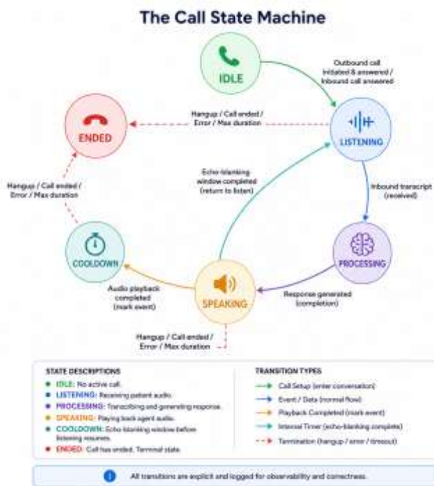
Figure 3: Finite-State Conversational Flow for Real-Time Voice Interaction
