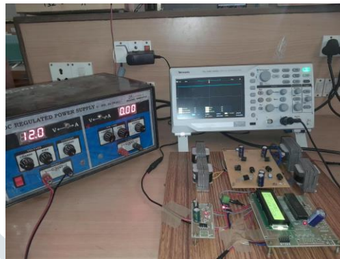
Fig. 6. Bench validation with a 0-30 V regulated DC supply replacing the PV module.
