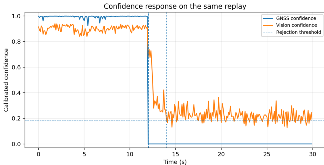
Figure 1. Calibrated GNSS and visual confidence on a representative concurrent-failure trajectory from the expanded held-out verification. The vertical markers indicate the GNSS fault at 12 s and the visual fault at 14 s.
