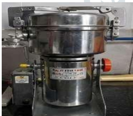
Figure 9 : Size Reduction by Chopping &amp; Sieving
