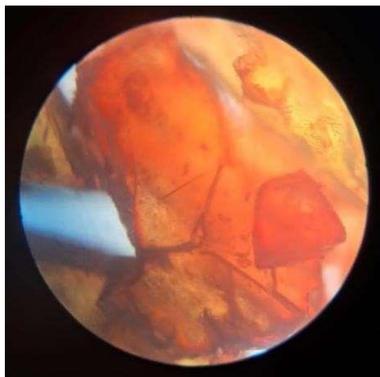
Fig. 2. Microscopic image of glitter fibres stained with Congo red.
