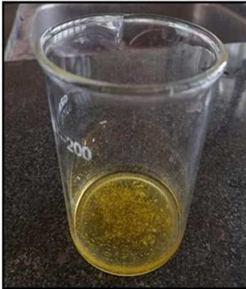
Fig. 4. Glitter dispersed in distilled water (turbidity test).
