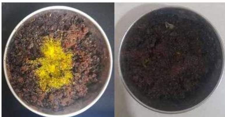
Fig. 6. Biodegradability of glitter in soil: before (left, Day 0) and after (right, 2–3 weeks).
