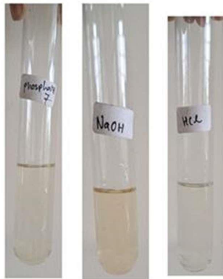
Fig. 5. Glitter immersed in solutions of different pH (colour fastness test).
