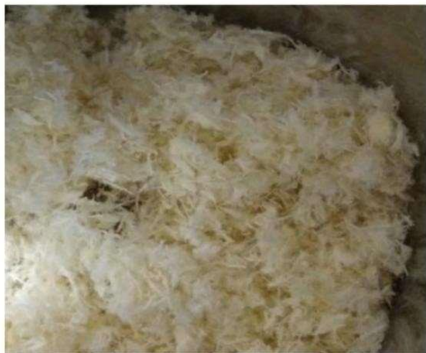
Fig. 1. Cellulose extracted from corn husk.
