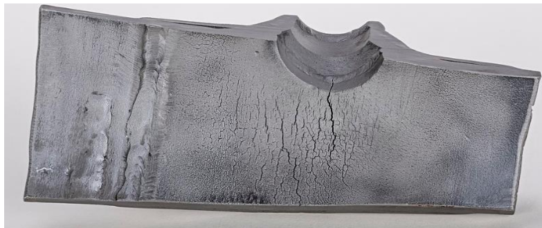
Figure (5): Stress Corrosion Cracking
