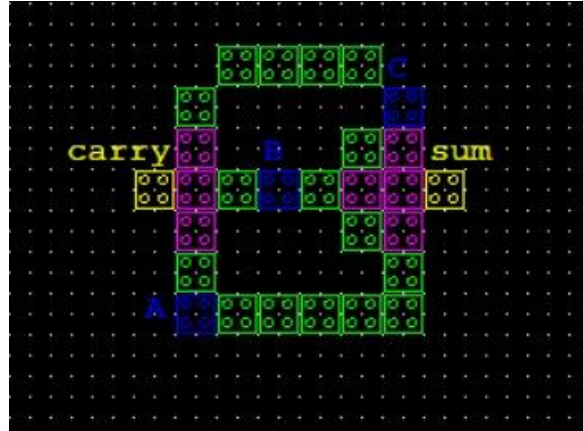
Fig. 27: FULL ADDER in QCA
