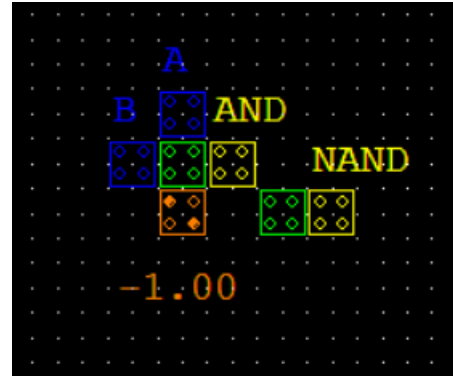
Fig.18: NAND gate in QCA
